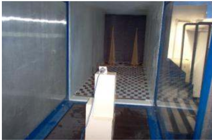
Fig. 7. Wind tunnel and instrumented scale model
