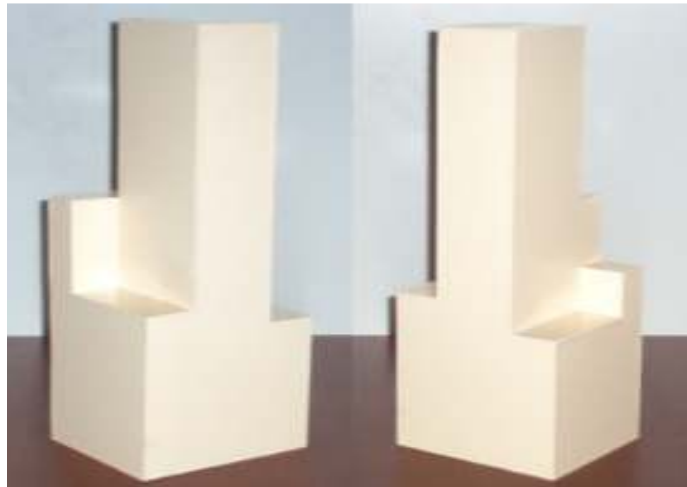
Fig. 6. Scale model made of PVC foamed material
