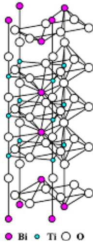
Fig. 1. Crystal structure of \text{Bi}_4\text{Ti}_3\text{O}_{12} [1]
