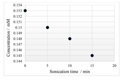
Fig. 5. Sonochemical decomposition of methyl orange in the absence of additives
