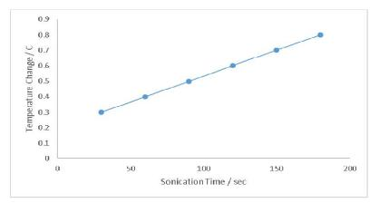
Fig. 4. The change of temperature with increasing sonication time
