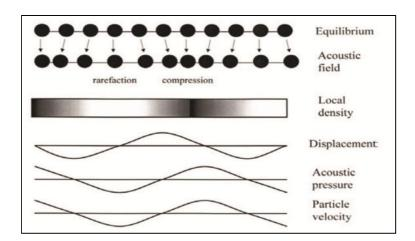
Fig. 2. Propagation of a one-dimensional ultrasound wave [C.E. Brennen, et al. Journal of fluid mechanics, 355 (1998) 255-283]
