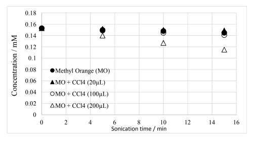
Fig. 9. Comparison of sonochemical decomposition of MO with and without different concentrations of CCl<sub>4</sub>
