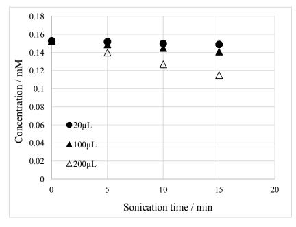
Fig. 8. Sonochemical decomposition of methyl orange in the presence of different concentrations of CCl<sub>4</sub>
