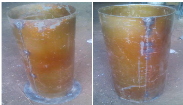
Fig. 2. Inner wall (left) and Outer wall (right) of combustion chamber
