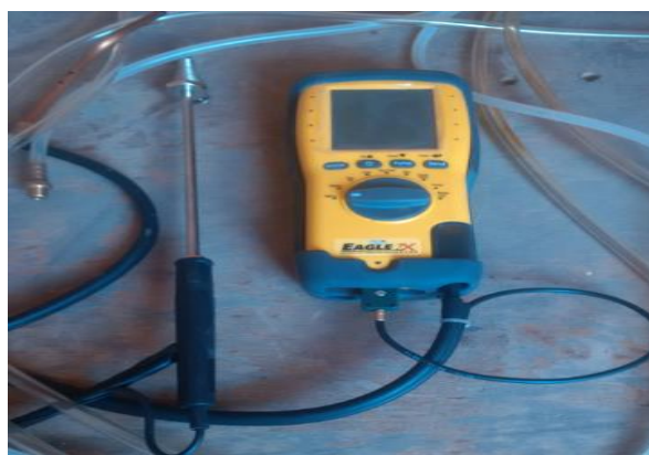
Fig. 4. Eagle 2X combustion analyzer
