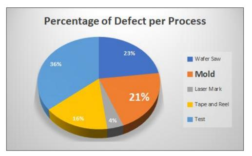
Fig. 3. Defect contribution per assembly process
