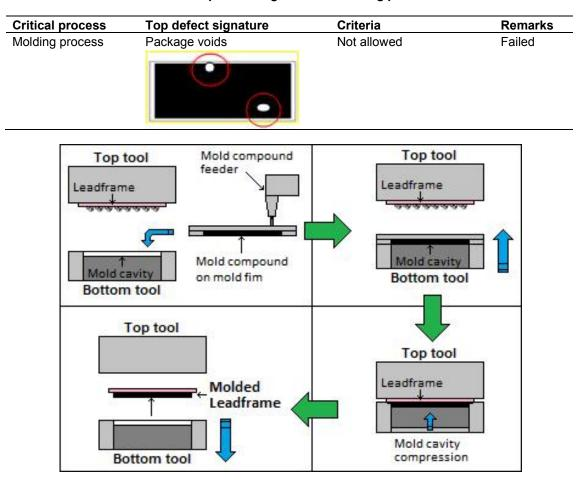
Fig. 5. Compression molding mechanism
