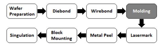
Fig. 2. Assembly process flow
