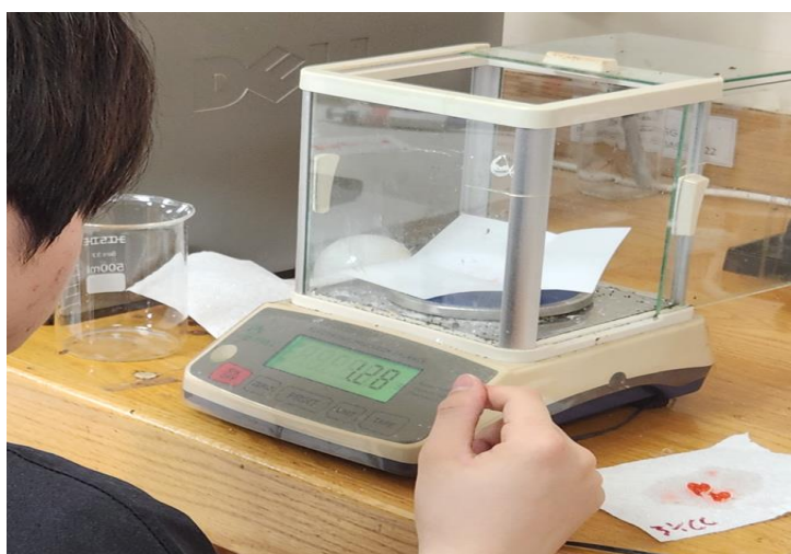
Fig. 4. Shows our method of measuring the bead weight using an electric balance
