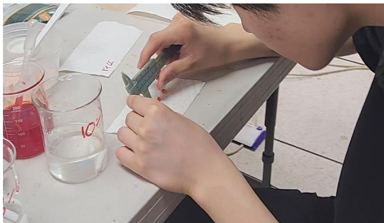
Fig. 3. Presents the methods of measuring bead size with a micrometer
