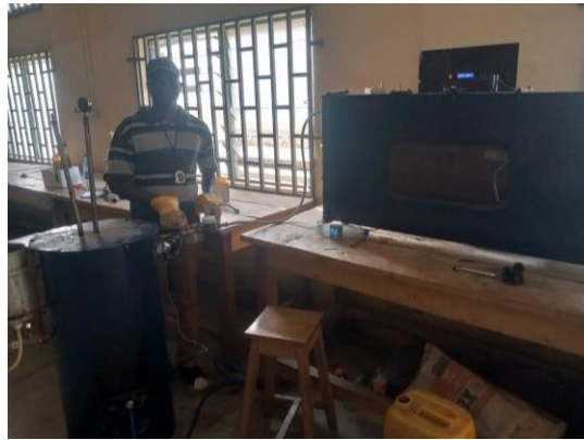
Plate 1. Steam Boiler, Sand Box and Condenser Set-Up for the Experiment
