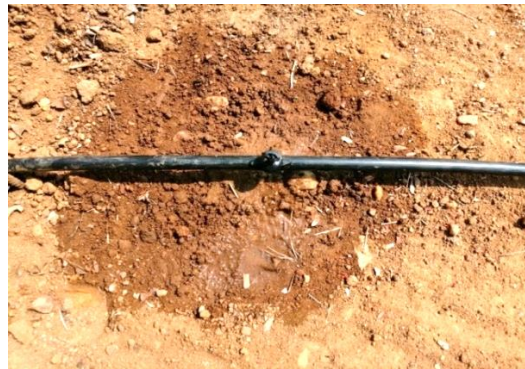
Fig. 3. Horizontal water zone radius of 4 lph dripper
