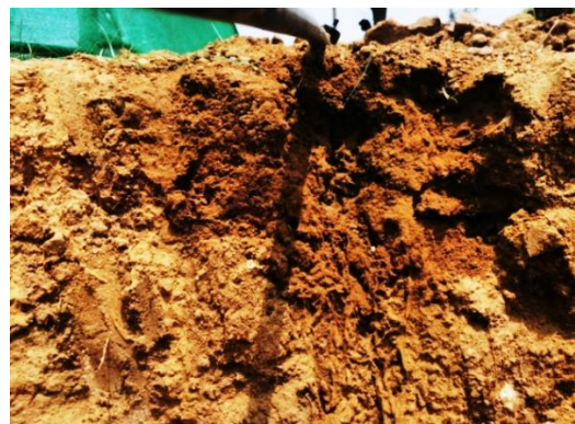
Fig. 4. Vertical water zone depth of 4 lph dripper
