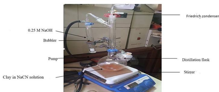
Fig. 2. Device for evaluating cyanide volatility
