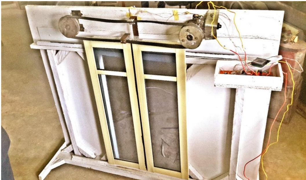
Fig. 9. Back view of the model of an automatic sliding door
