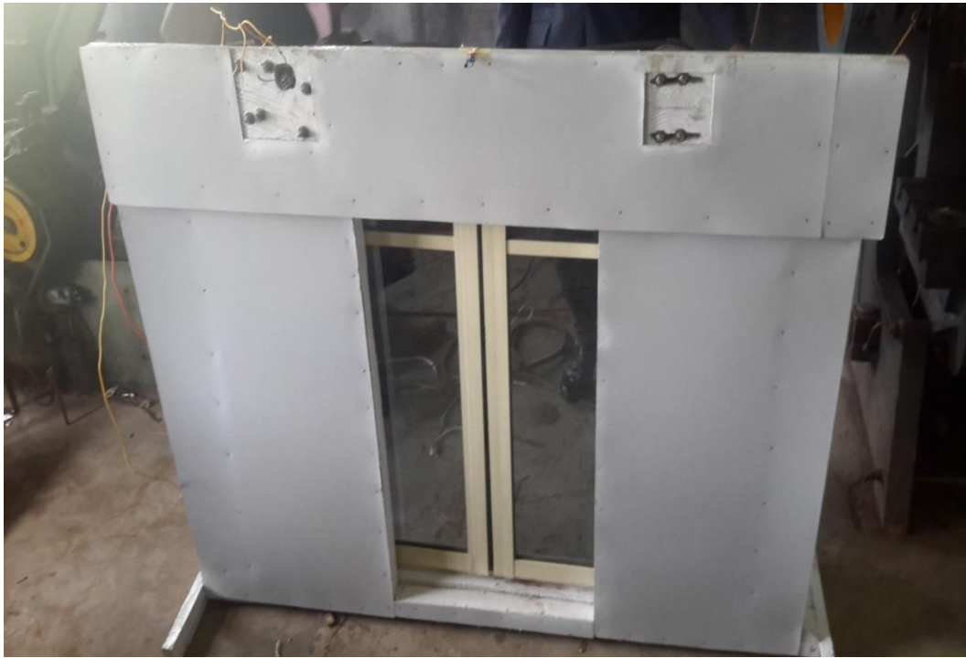
Fig. 8. Front view of the model of an automatic sliding door
