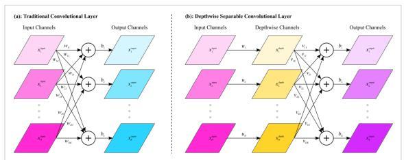
**Figure 8.** Visualization of convolutional layers. (a) Traditional convolutional layer where output channels are sums of biases and convolutions of weights with input channels. (b) Depthwise separable convolutional layer where depthwise convolutions compute one convolution with weights for each input channel. Output channels are sums of biases and pointwise convolutions weights with depthwise channels.
