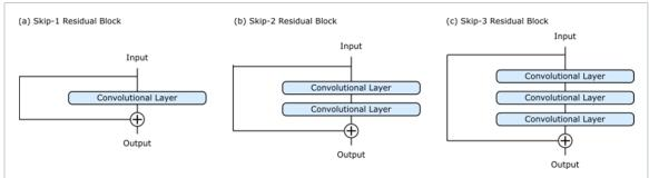
**Figure 10.** Residual blocks where (a) one, (b) two, and (c) three convolutional layers are skipped. Typically, convolutional layers are followed by batch normalization then activation.
