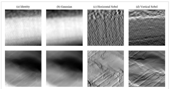
**Figure 9.** Two 96  $\times$  96 electron micrographs (a) unchanged, and filtered by (b) a 5  $\times$  5 symmetric Gaussian kernel with a 2.5 px standard deviation, (c) a 3  $\times$  3 horizontal Sobel kernel, and (d) a 3  $\times$  3 vertical Sobel kernel. Intensities in (a) and (b) are in [0, 1], whereas intensities in (c) and (d) are in [-1, 1].
