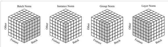
**Figure 7.** Visual comparison of various normalization methods highlighting regions that they normalize. Regions can be normalized across batch, feature and other dimensions, such as height and width.
