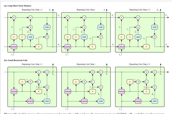
Figure 13. Architectures of recurrent neural networks with (a) long short-term memory (LSTM) cells, and (b) gated recurrent units (GRUs).
