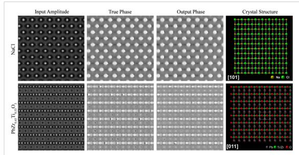
**Figure 4.** Example applications of a DNN to reconstruct phases of exit wavefunction from intensities of single TEM images. Phases in  $[-\pi,\pi)$  rad are depicted on a linear greyscale from black to white, and Miller indices label projection directions. This figure is adapted from our earlier work [349] under a Creative Commons Attribution 4.0 [73] license.
