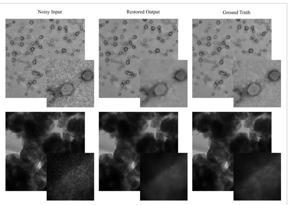
**Figure 1.** Example applications of a noise-removal DNN to instances of Poisson noise applied to  $512 \times 512$  crops from TEM images. Enlarged  $64 \times 64$  regions from the top left of each crop are shown to ease comparison. This figure is adapted from our earlier work [72] under a Creative Commons Attribution 4.0 [73] license.
