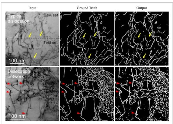
**Figure 3.** Example applications of a semantic segmentation DNN to STEM images of steel to classify dislocation locations. Yellow arrows mark uncommon dislocation lines with weak contrast, and red arrows indicate that fixed widths used for dislocation lines are sometimes too narrow to cover defects. This figure is adapted with permission [287] under a Creative Commons Attribution 4.0 [73] license.
