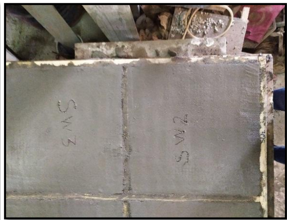
d. Shows leveling the mortar surface
