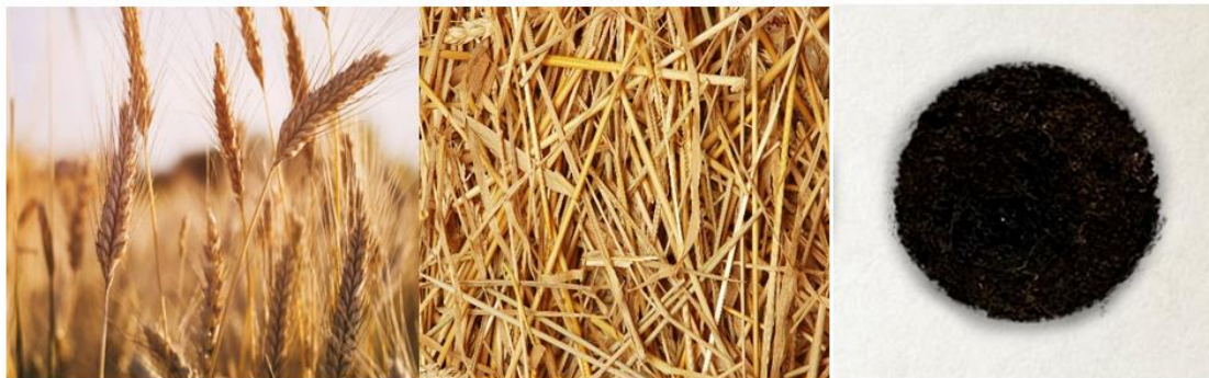
Fig. 2. a) Wheat crop b) Wheat Straw separation c) Wheat straw ash burning at 800°C for 30min
