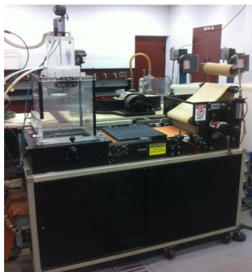
Fig. 3. MK Systems Inc. dynamic sheet former [29]
