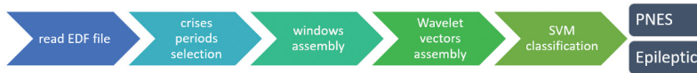
Figure 3. Process steps used to differentiate between PNES and ES in EEG signals.
