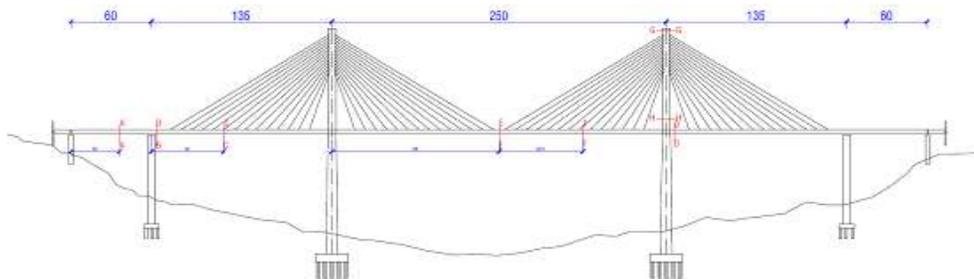
Fig. 6. The test section layout diagram (unit: m)
