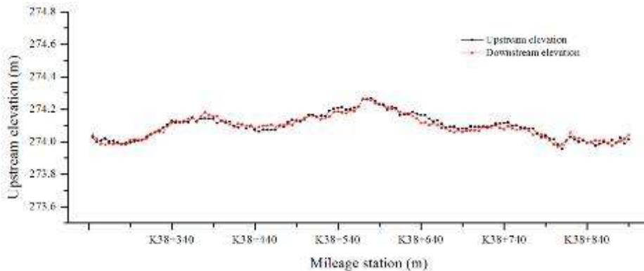
Fig. 3. The measured line shape of the girder
