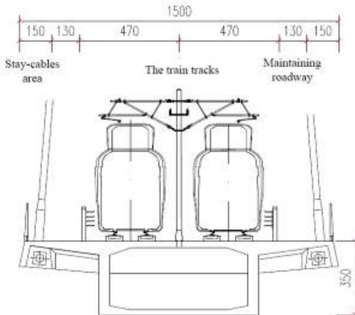
Fig. 2. Cable-stayed bridge cross section diagram (unit: cm)
