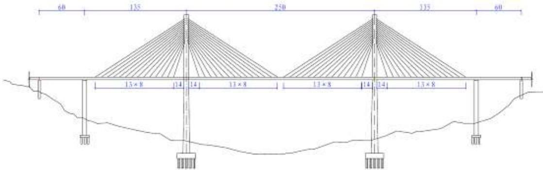
Fig. 1. Cable-stayed bridge elevation layout (unit: m)
