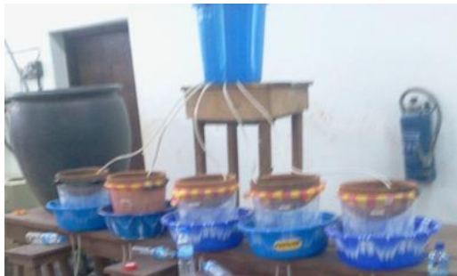
Fig. 2. Laboratory set-up for flow rate test on the ceramic filters
