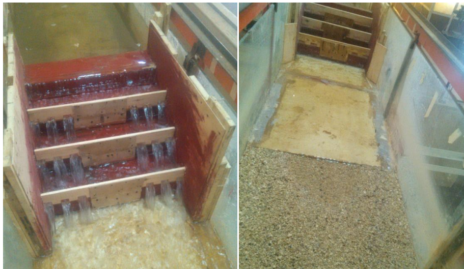
Photo 2. The openings in breakers and downstream divergent angle in flume
