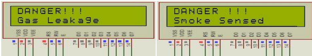
Figs. 7c and 7d. Output from display when at least one switch in the smoke detection sensor group is activated [15]
