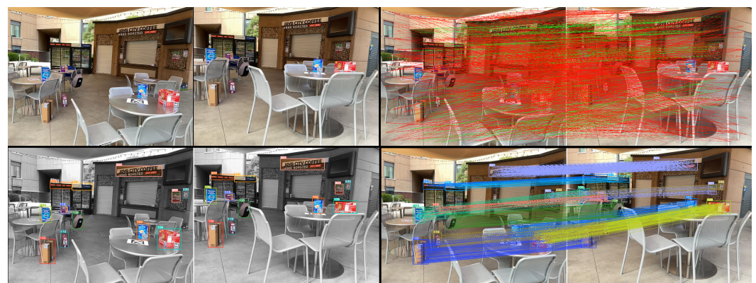
Figure 1. Comparison of the standard matching and our object-oriented matching approach on whole images. (Top Left): The picture on the left is the reference frame, and the right is the query frame captured by a robot camera at the Javacity Cafe. (Top Right): The standard ORB real-time matching from the reference to query. (Bottom Left): The unique objects are detected by Yolov5 on both frames with bounding boxes in various colors. (Bottom Right): Our object-oriented compact feature matches from reference to query frame by reusing features stored in object detectors.
