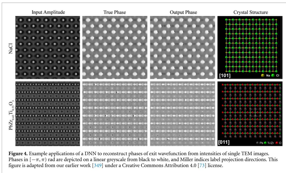
**Figure 4.** Example applications of a DNN to reconstruct phases of exit wavefunction from intensities of single TEM images. Phases in  $[-\pi, \pi]$  rad are depicted on a linear greyscale from black to white, and Miller indices label projection directions. This figure is adapted from our earlier work [349] under a Creative Commons Attribution 4.0 [73] license.
