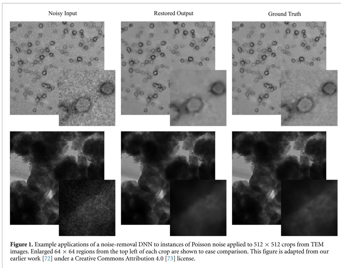
**Figure 1.** Example applications of a noise-removal DNN to instances of Poisson noise applied to  $512 \times 512$  crops from TEM images. Enlarged  $64 \times 64$  regions from the top left of each crop are shown to ease comparison. This figure is adapted from our earlier work [72] under a Creative Commons Attribution 4.0 [73] license.
